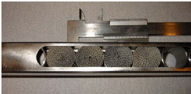
Fig. 1. Catalysts inside an ageing rack.
